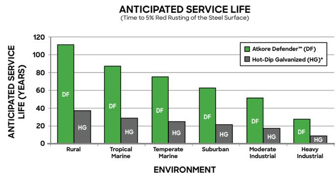
\*Hot-Dip Galvanized per ASTM A123 and A153 coating service life as specified within the North American Metal Framing Industry
